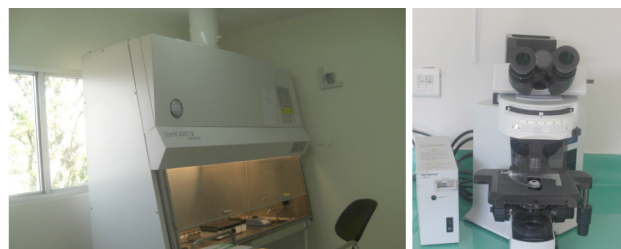
Class II bio-safety Cabinet and a fluorescent microscope used in the mycology laboratory.
